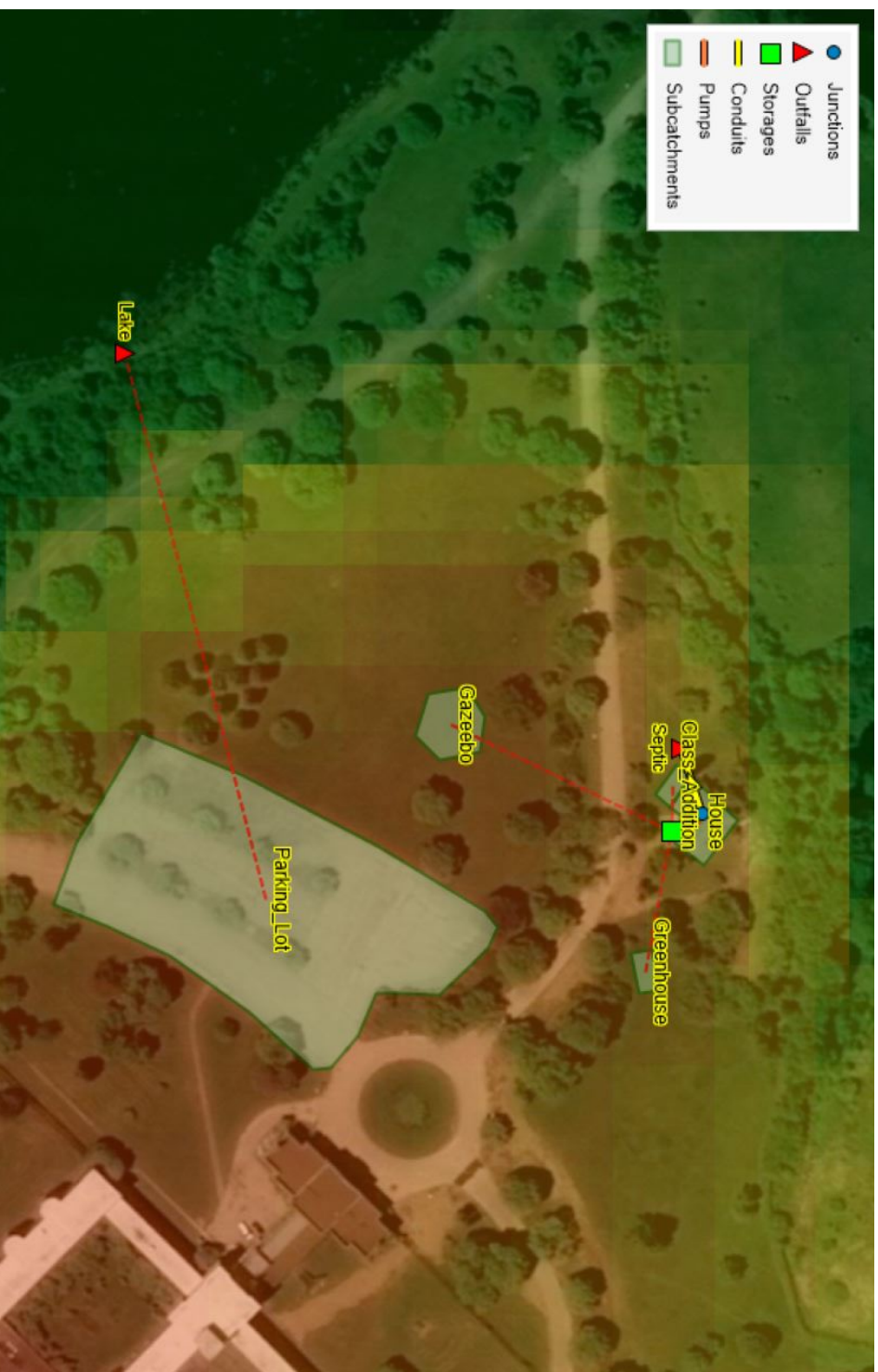
Figure H-6: PCSWMM Model Layout including aerial imagery and DEM overlay where green is lower elevation and red is higher (range 315m to 322m).
