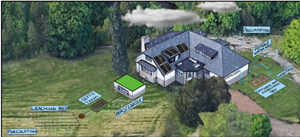
Figure 4-3: Proposed 'One Water' system layout including water flow pathways.
