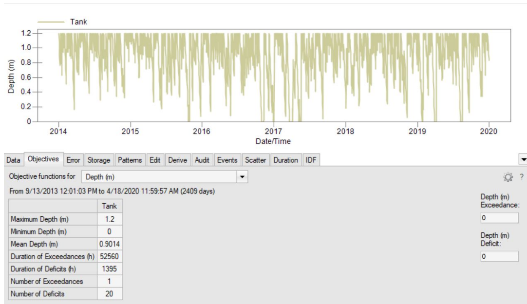
Figure H-8: Plot of tank levels during model simulation years 2014 to 2020 for the final design scenario.
